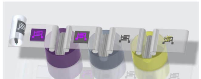
Fig. 2 Schematic of PRL/IDT/Hydrothermal procedure
