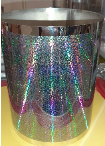
Figure 3: Laser welded nickel plate forms a sleeve.
