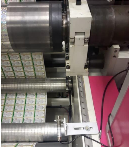
Figure 5: Measuring the temperature of the black stripe at the end of the imprinting cylinder by an IR sensor (below middle on the photo).
