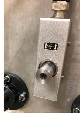
Figure 2: Load cell to measure web tension
